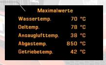
Specifies the maximum value of the current drive; When the switch off the ignition deletes these values
